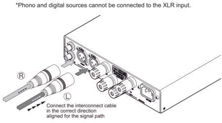
for better sound quality. Pinning: 1=Ground, 2=Hot, 3=Cold. \*Phono and digital sources cannot be connected to the XLR input
